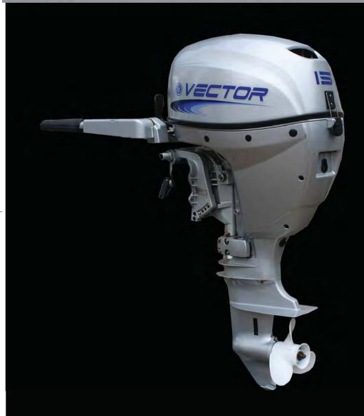
Models F15S/L & ES/EL Max. Output (kw) Max Operating Range 4500-5500 Stroke Cylinders Displacement (cm3) 323 Bore x Stroke (mm) 59 x 59 Compression Ratio 9.9:1 Dimensions (mm) shortshaft 1000x427x1080 Dimensions (mm) longshaft 1000x427x1207 Weight (kg) 49 & 52 Gear Ratio 2.08:1 Gear Shift Positions F-N-R Ignition System CDI Cooling System Water-cooling Manual or Electric Starting System Control System Tiller or Remotes Standard 12 Fuel Tank Capacity (L) Option 24
